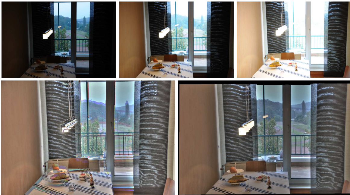
Figure 6.13: Freehand HDR imaging of another indoor scene ( Room ). First row, from left to right: (a)–(c) Image 1, 2 and 3 of the exposure series (3 images, 1024 \times 680 pixels, exposure times between 1/60 and 0.3 seconds). Second row, from left to right: (c) Resulting tone mapped HDR image without alignment. (d) Same using our proposed alignment method.
