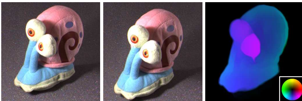
Figure 1.1: Optic flow estimation. From left to right: (a) First image. (b) Second image. (c) Computed flow field using our approach in [10, 11], visualised using the colour code shown in the inset.
