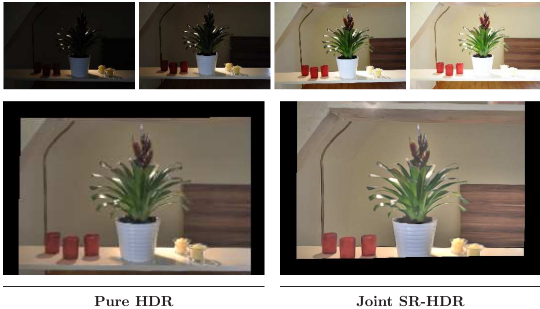
Figure 6.18: Comparing a pure HDR to a joint SR-HDR result on an indoor scene. First row, from left to right: (a) – (d) Images 1, 3, 6 and 8 of the exposure series (8 images, 268 \times 178 pixels, exposure times between 1/200 and 1/8 seconds.) Second row, from left to right: (d) HDR result after aligning the exposure series with our proposed technique. (e) SR-HDR result using our proposed approach. (same alignment, \vartheta = 0.6 ).
