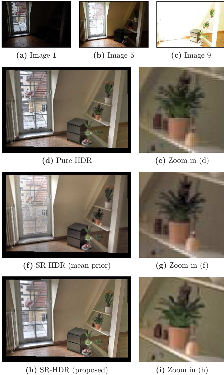
Figure 6.16: Joint SR-HDR reconstruction on a real world exposure series. First row, from left to right: (a) – (c) Images 1, 5 and 9. Second row, from left to right: (d) Upsampled HDR reconstruction. (e) Zoom in (d). Third row, from left to right: (f) SR-HDR result of [CPK09, GG06] (quadratic data term, mean prior, \vartheta=5.0, \tau=0.1 , 25 iterations). (g) Zoom in (f). Fourth row, from left to right: (h) Result of proposed method ( \vartheta=0.3, s=8, \rho_1=0.4, \rho_2=0.2, \tau=0.5 , 1000 iterations). (i) Zoom in (h).
