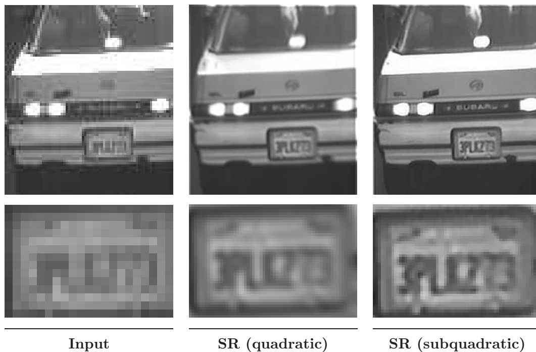
Figure 6.15: Super-resolution example. First row, from left to right: (a) One of the input images (64 images, 72 \times 121 pixels, taken from http://users.soe.ucsc.edu/~milanfar/software/sr-datasets.html ). (b) Super-resolution result using a quadratic data term and a homogeneous smoothness term ( \vartheta = 1.0 ). The used zoom factor was z = 3 . (c) Same using a L_1 data term and a TV smoothness term ( \vartheta = 0.7 ). Second row, from left to right: (d)–(f) Zooms in (a)–(c).
