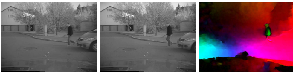
Figure 1.2: Optic flow for driver assistance. From left to right: (a) First image of a sequence taken out of a car [WPZ + 08]. (b) Second image. (c) Optic flow field computed using our approach in [10, 11]. Note that the pedestrian is easily distinguishable.
